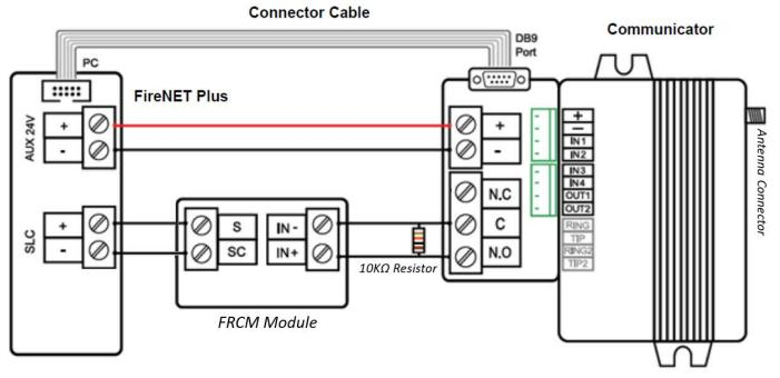
\*The Pathway Pro trouble relay does not change states on power up. There is a delay of 5-8 minutes before the relay activates on a loss of communication trouble.
